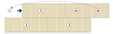
Dura SlimStack 12 panels should be butt-joined horizontally. This will maintain the SlimStack pattern.
