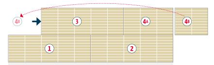
Dura SlimStack 10 panels should be butt-joined horizontally. This will maintain the SlimStack pattern.
