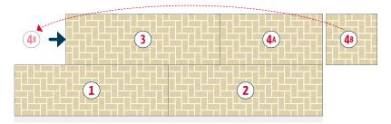
Panels should be butt-joined horizontally. Half bricks at ends of each panel will align to create full bricks.
