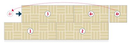
Panels should be butt-joined horizontally. Half bricks at ends of each panel will align to create full bricks.
