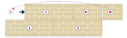
Panels should be butt-joined horizontally. Half bricks at ends of each panel will align to create full bricks.
