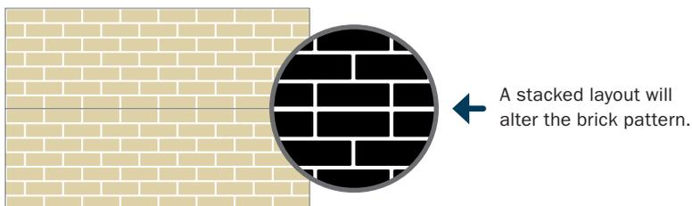
Dura Standard 214 panels should be butt-joined horizontally. Half bricks will align to create full bricks.
