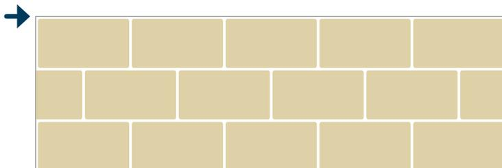
*Dura CinderBlock 3* looks best installed using an offset layout on alternate rows.
