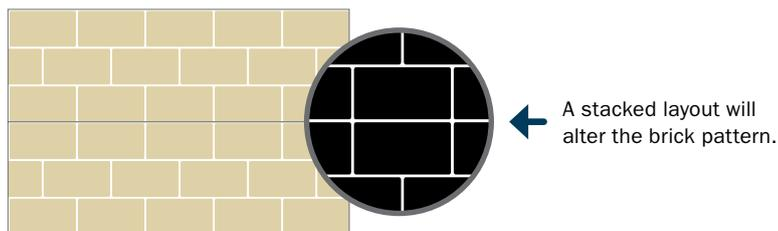
*Dura CinderBlock 3* panels should be butt-joined horizontally. Half bricks will align to create full bricks.
