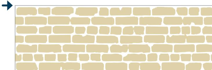
Dura Rustic looks best installed using an offset layout on alternate rows.
