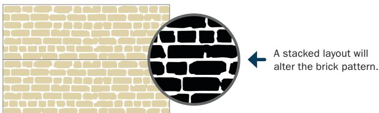
Dura Rustic panels should be butt-joined horizontally. Half bricks will align to create full bricks.
